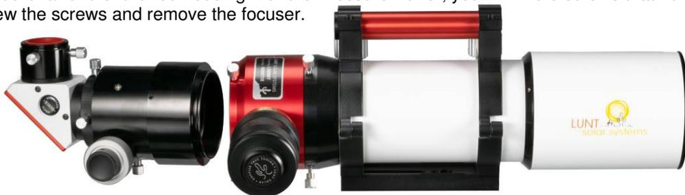
Now place the DSII module to the point where previously the focuser was and fix it with the 3 screws.
