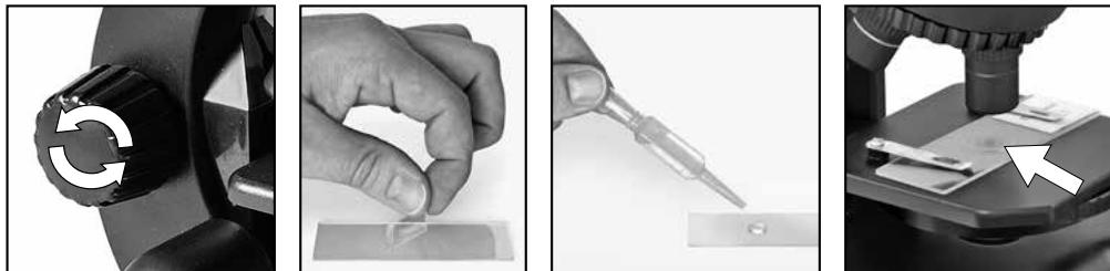
For normal observation, place the microscope in a bright location (near a window or desk lamp, for example). Turn the focus knob (2) to the upper stop, and set the objective turret (3) to the lowest magnification.
