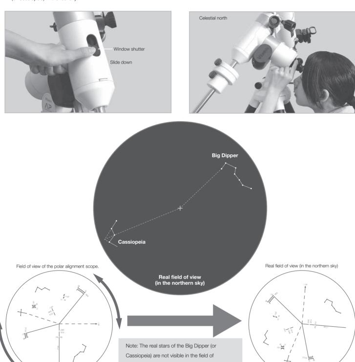
The patterns of the Big Dipper and Cassiopeia on the reticle are positioned to correspond to the real sky. They are used as a guidepost to know the turning direction of the polar alignment scope's reticle. The locations of the Big Dipper and Cassiopeia on the reticle have no relation to the location of Polaris, Delta UMi and 51 Cep on the reticle.
