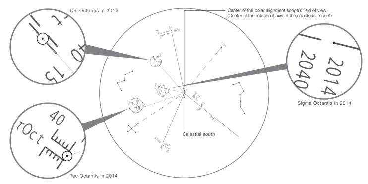
As an illustration here, Sigma Octantis is set to the edge of the line on the side of 2014, and both Tau and Chi Octantis are set to the middle of the curved lines of the position scale at the protruded edge on the side of 15 respectively. (In case of the year 2014)
