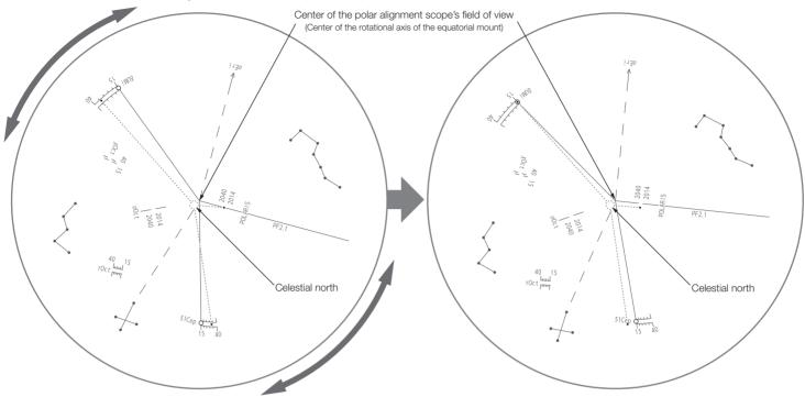
Since there is no mark that points at the North Celestial Pole, you need to match the polar axis of your AP equatorial mount with the N.C.P using the conspicuous polar star and two stars in the same area of the sky. This is called polar alignment.
