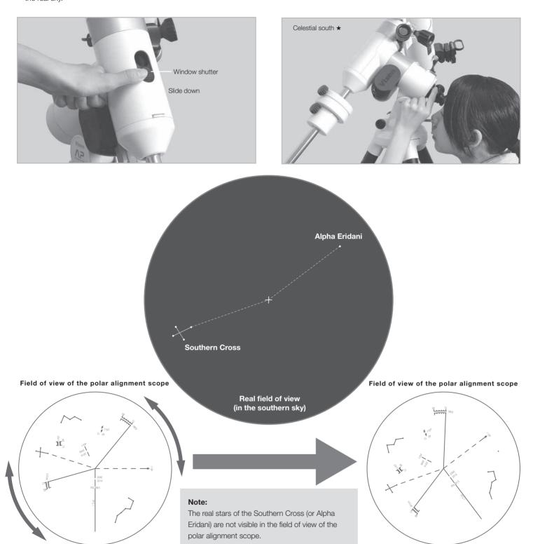
Both the Southern Cross and Alpha Eridani on the reticle are positioned to correspond to the real sky. They are used as a guidepost to know the turning direction of the polar alignment reticle. The locations of the Southern Cross and Alpha Eridani on the reticle have no relation to the locations of the Octantis stars on the reticle.
