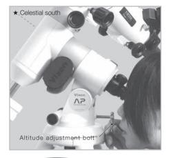
Correcting the position of Sigma Octantis with the altitude adjustment bolt and azimuth adjustment knobs
