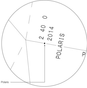
As Polaris shifts to the designated position on the reticle, both Delta UMi and 51 Cep come close to their own designated position scales respectively. While looking into the eyepiece of the polar alignment scope, turn the polar alignment scope body so that each of the position scale for Delta UMi and 51 Cep come to the closest to actual Delta UMi and 51 Cep respectively.
