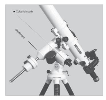
Open the round window on the declination body by sliding down the shutter of the window. While looking into the polar alignment scope, turn the polar alignment scope body so that the engraved Southern Cross (or Alpha Eridani) on the reticle directs the Southern Cross (or Alpha Eridani) in the real sky.
