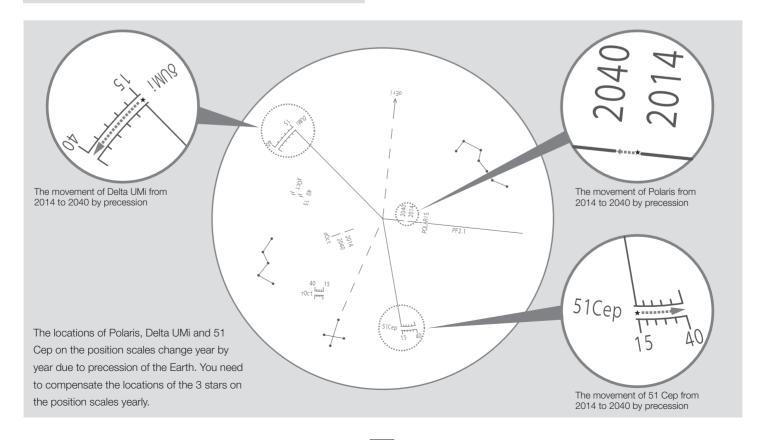
6 While looking into the eyepiece of the polar alignment scope, turn the altitude adjustment bolt and azimuth adjustment knobs so that Polaris comes to the gap between the two segments of the lines marked 2014 and 2040.
