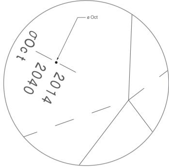
As Sigma Octantis shifts to the designated position on the reticle, both Tau Octantis and Chi Octantis come close to their own designated position scales respectively. While looking into the eyepiece of the polar alignment scope, turn the polar alignment scope body so that each of the position scale for Tau Octantis and Chi Octantis come to the closest to actual Tau Octantis and Chi Octantis respectively.
