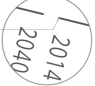
Repeat the procedures 5 and 6 until Sigma, Tau and Chi Octantis come to the proper locations on the designated position scales respectively. Tighten the azimuth adjustment knobs at both sides to finish the polar alignment.
