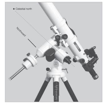
Open the round window on the declination body by sliding down the shutter of the window. While looking into the polar alignment scope, turn the polar alignment scope body so that the engraved Big Dipper (or Cassiopeia) on the reticle matches the Big Dipper (or Cassiopeia) in the real sky.
