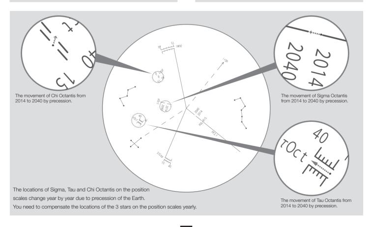
While looking into the eyepiece of the polar alignment scope, turn the altitude adjustment bolt and azimuth adjustment knobs so that Sigma Octantis comes to the gap between the two segments of the lines marked 2014 and 2040.
