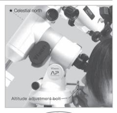
Correcting the position of Polaris with the altitude adjustment bolt and azimuth adjustment knobs
