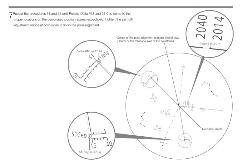
As an illustration here, Polaris is set to the edge of the line on the side of 2014, and both Delta UMI and 51 Cep are set to the middle of the curved lines of the position scale at the protruded edge on the side of 15 respectively. (In case of the year 2014)
