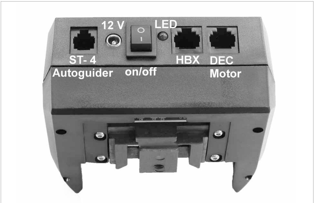
Fig. 1b: Control-Panel of RA motor
