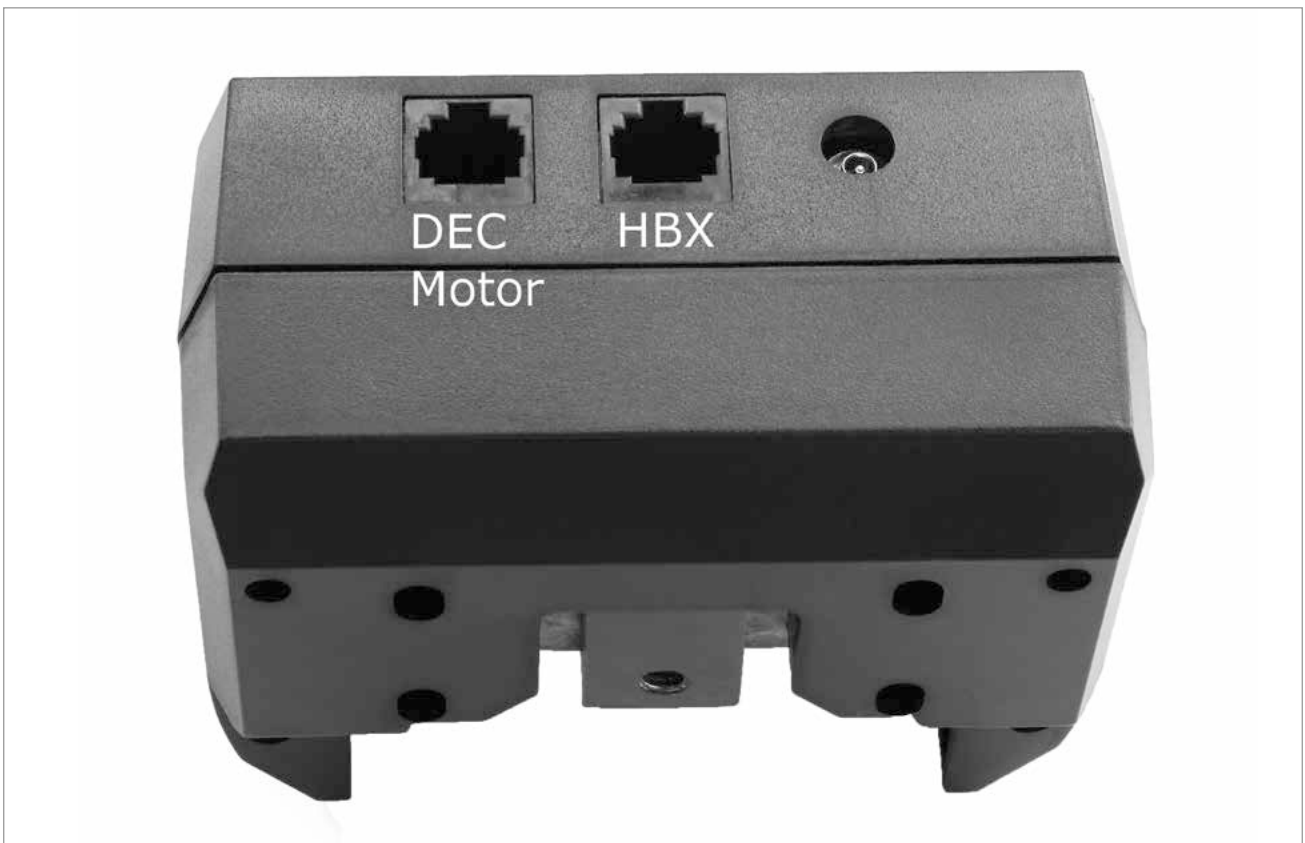
Fig. 1c: Control-Panel of DEC Motor
