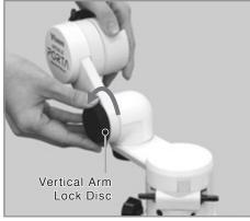
2 While holding the altitude multi-arm, loosen the horizontal arm lock disc to set up the orientation of the altitude multi-arm to your desired direction.
