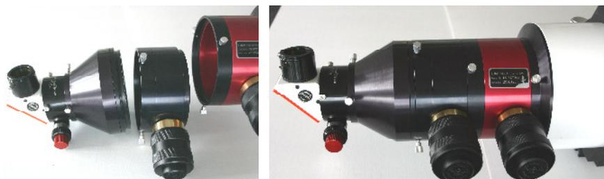
The user may rotate the DSII into any position. Snug the allen head screws or aluminum thumbscrews onto the module and fasten it in place. Now the installation of the DSII module at the LS152THa telescope is finished.
