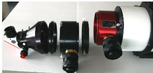
Thread the cone/focuser assembly onto the male adapter and thread the female adapter onto the red LS152THa pressure tune assembly.
