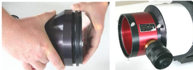
Attach the DSII unit to the red LS152THa pressure tune assembly. Then attach the cone/focuser to the DSII unit.
